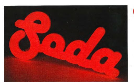
**NOTE ON LED USAGE:** GemLite Formed Channel Letters are UL-recognized components for LED installations. The renewable resource plastics used in the faces and cans have a flammability rating of 1 and fire rating of 94HB, and can be used with virtually any low-voltage, low-profile lighting system that does not require a metal can for a heat sink. These letters are not for use with any neon or other lighting system of greater than 24V.
