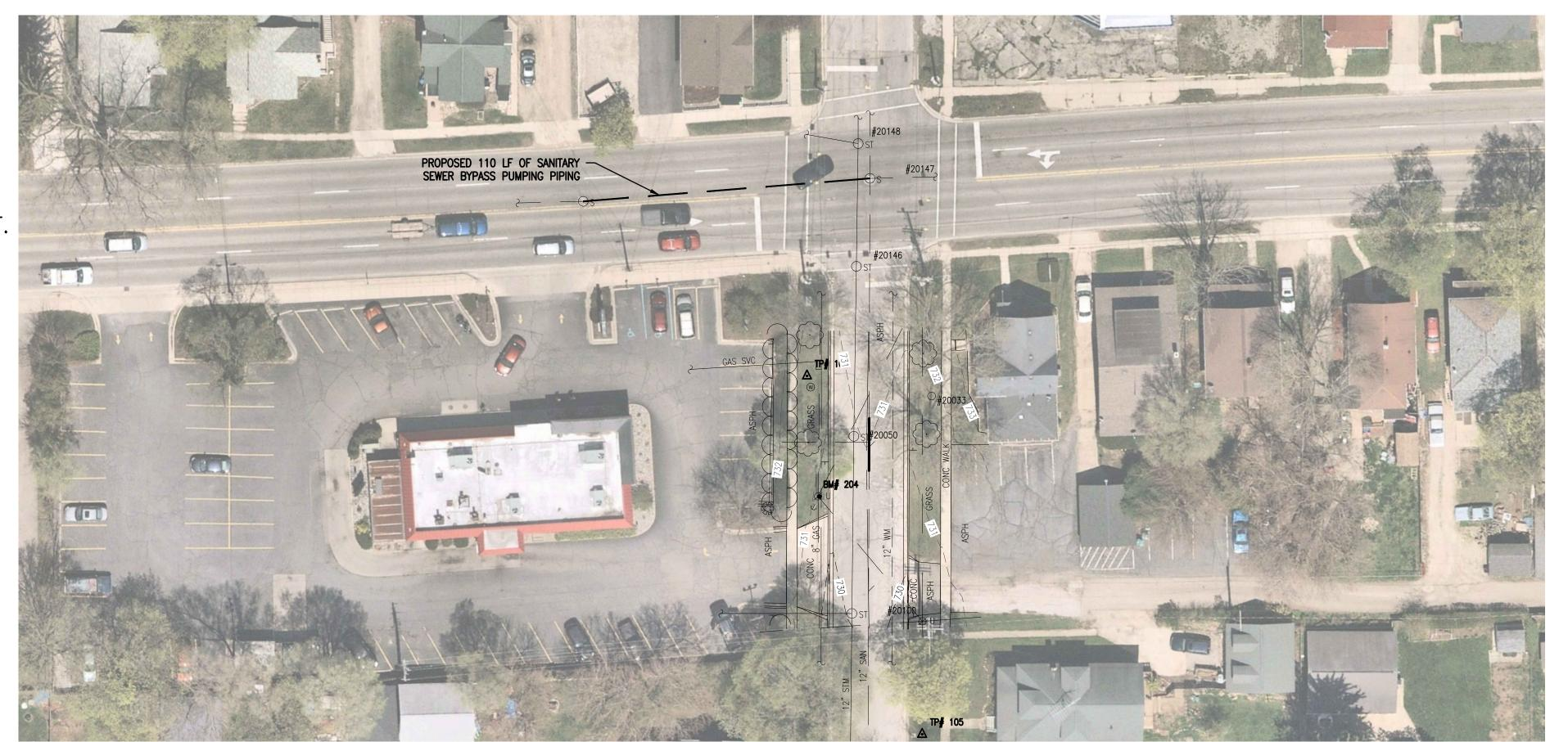
SANITARY SEWER BYPASS PUMPING PLAN SCALE: 1"=30"
