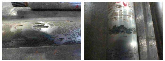
Pitting/Corrosion of shaft
