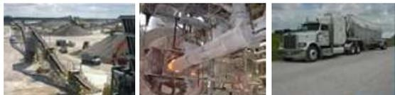
Quicklime comes from limestone that is mined from the ground, crushed to size, heated in a kiln, and then transported by truck to the Treatment Facility
